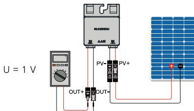
An actual reading of  $1\pm0.1$  V is considered to be within normal range due to the difference in the accuracy of the measurement instrument. Replace the optimizer if the measurement is beyond this range.
