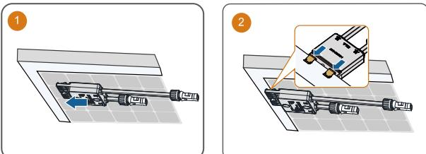
Please ensure that the optimizer is installed facing the back of the module. Otherwise, the clip may be damaged.
